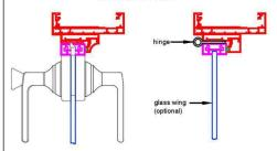
The panels of the Ocean - Style doors are 6 - 8 millimeter tempered glass. A narrow, decorative frame covers the sides. Panel can also be applied as half - wood and half - glass. The desired door and glass accessories can be easily applied. Usage Areas: Offices, restaurants, toilets, schools, and universities, hospitals, etc.
