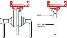
The panels of the Atmosphere - Style doors are completely made of transparent glass. The desired glass and door accessories can be easily applied. The panels can be modelled and be used with different colored glasses. As a standard, it is produced with the 10 - millimeter security glass. If desired, the glass in different width can be applied. Usage Areas: Offices, restaurants, toilets, schools, universities, hospitals, showrooms, etc.
